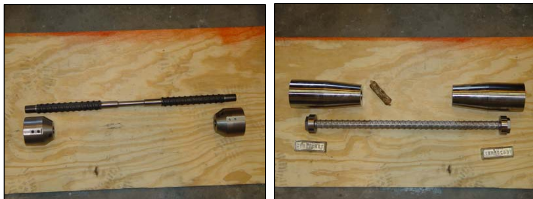
Figure 4. Machined (left) and as-rolled (right) reinforcement bars.
