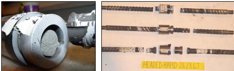
Figure 21. Posttest photos of upset head specimens tested at rapid strain rate.
