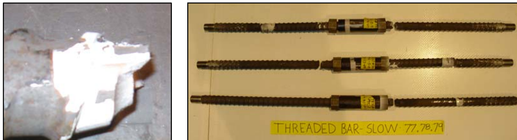
Figure 41. Posttest photos of threaded bar specimens tested at slow strain rate.
