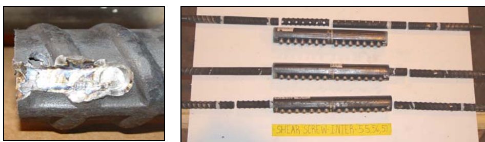
Figure 31. Posttest photos of shear screw specimens at the intermediate strain rate.
