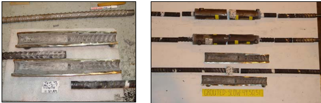
Figure 23. Posttest photos of grouted sleeve specimens tested at the slow strain rate.
