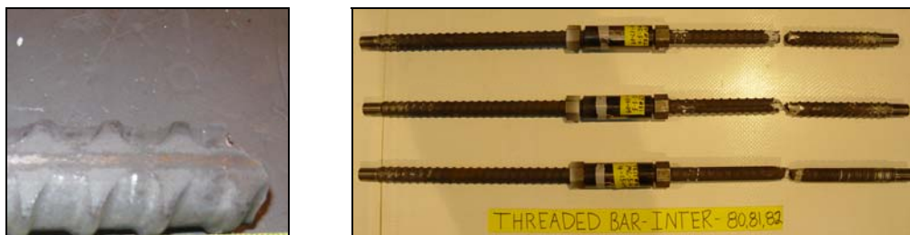
Figure 43. Posttest photos of threaded bar specimens tested at intermediate strain rate.
