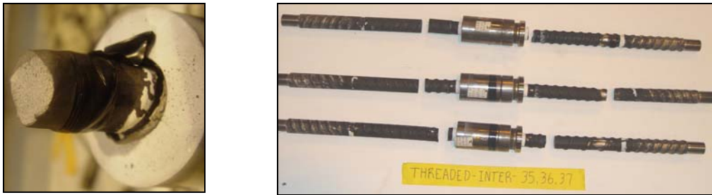
Figure 37. Posttest photos of taper threaded specimens tested at intermediate strain rate.
