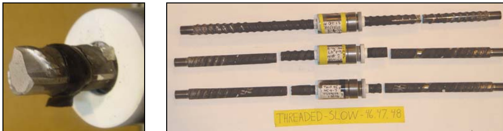
Figure 35. Posttest photos of taper threaded specimens tested at the slow strain rate.
