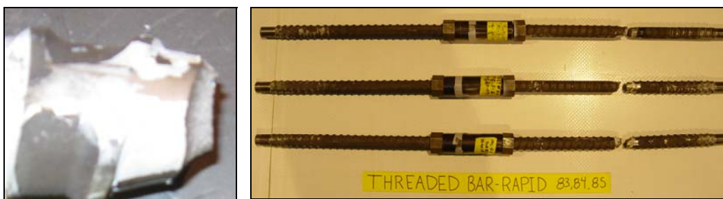
Figure 45. Posttest photos of threaded bar specimens tested at rapid strain rate.
