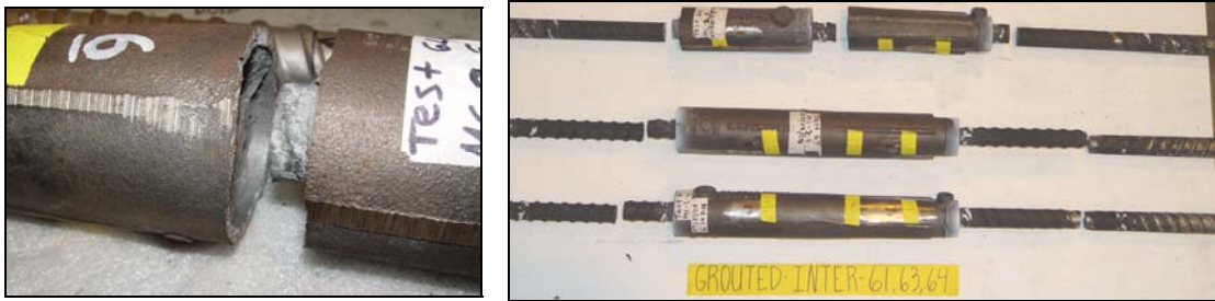
Figure 25. Posttest photos of grouted specimens tested at the intermediate strain rate.
